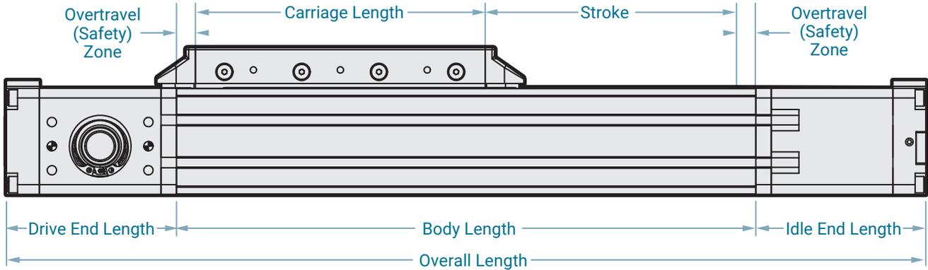
There are two common ways to determine the *Body Length* for an actuator. The first is to start with the *Overall Length* and subtract, the second is to start with the *Stroke* and add. The easiest option is to start with the *Overall Length* and subtract the *Drive End Length* and the *Return End Length* to find the *Body Length*. This is most commonly done when the actuator must fit inside of an enclosed cabinet and the engineer's goal is to obtain the maximum amount of *Stroke* possible.
